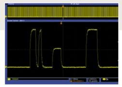
Since an oscilloscope can store only a limited number of samples, the waveform duration (time) will be inversely proportional to the oscilloscope's sample rate. **Time Interval = Record Length / Sample Rate**
