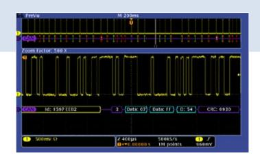
Oscilloscopes with record lengths in the millions of points can show thousands of screens worth of signal activity, essential for examining complex waveforms. Placing **marks** on the waveform assists in latency measurements on a CAN bus, for example.
