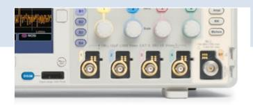
A mixed domain oscilloscope not only offers analog and digital channels, like an MSO, but also includes a dedicated RF input channel that behaves like a spectrum analyzer.
