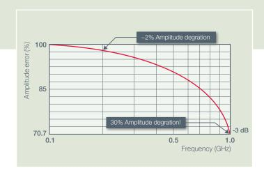
Bandwidth is defined as the frequency at which a sine-wave input signal is attenuated to 70.7% of its true amplitude (the -3 dB or 'half-power' point, shown here for a 1 GHz scope).
